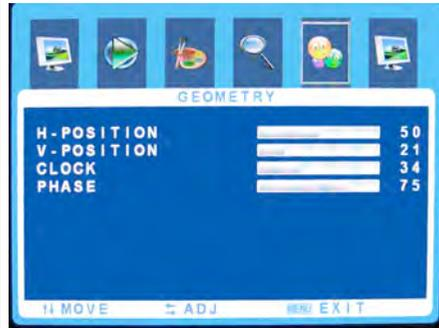
**H-POSITION :** Moves image horizontally on screen either left (<) or right (>).
