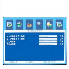
**H-POSITION:** Moves image horizontally on screen either left (<) or right (>).
