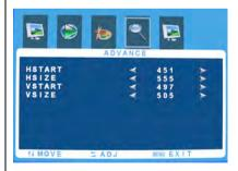
Press< or > for desired adjust parameter option until satisfactory value is achieved ,when VGA signals are received ,the automatic modes is used for parameter adjustment.
