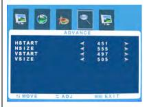
Press< or > for desired adjust parameter option until satisfactory value is achieved ,when VGA signals are received ,the automatic modes is used for parameter adjustment.
