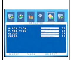
**H-POSITION:** Moves image horizontally on screen either left (<) or right (>).
